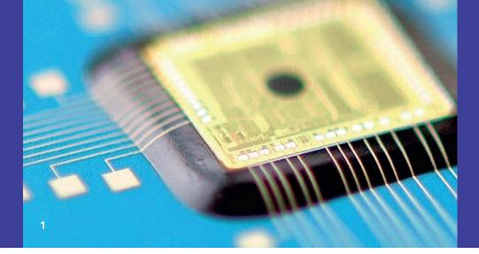
Fraunhofer IKTS possesses unique know-how in the preparation and processing of optimized inks, especially for meeting the special requirements of ceramic parts with respect to co-sintering and shrinkage behavior. These inks are composed of organic components (binders, dispersants, and solvents) and solid particles (e.g., metals, glasses, or oxides).
